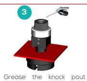
Grease the knock pout punch and the sheet plate in order to simplify the cut.
